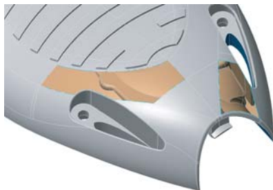
Surface repair of corrupt or missing surfaces ready for closing to a solid.
