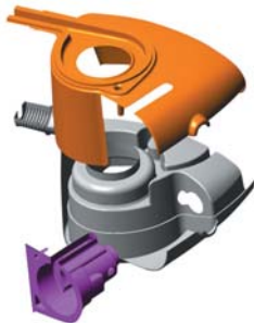
Upper and lower halves of a component for the toy industry split with VISI-Split.
